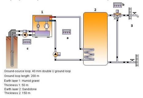
*Figure 4: Hydraulic diagram for domestic hot water preparation with geothermal heat pump systems.*
