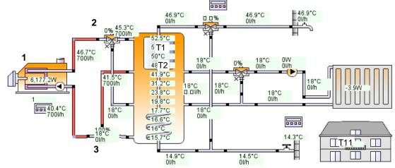
Figure 7: Operation mode domestic hot water.
