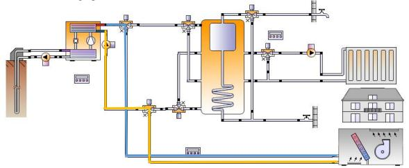
*Figure 11: Hydraulic diagram for domestic hot water, space heating and space cooling with a reverse working ground source heat pump.*
