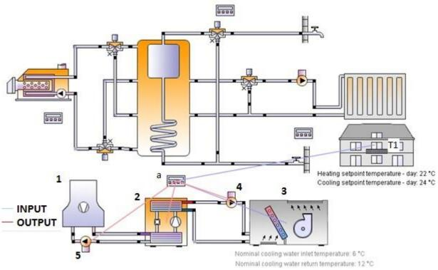
Figure 10: Hydraulic diagram with control system for domestic hot water, space heating and space cooling.
