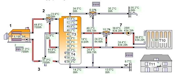
Figure 8: Operation mode space heating.
