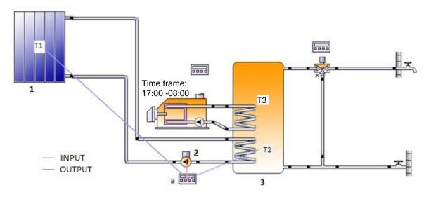
*Figure 3: Hydraulic diagram for domestic hot water preparation with solar thermal support.*
