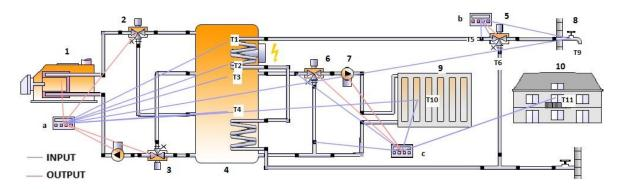
Figure 6: Hydraulic diagram with control system for heating and domestic hot water preparation.
