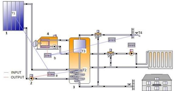
Figure 9: Hydraulic diagram for domestic hot water and heating preparation with solar thermal support.
