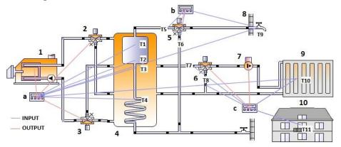
Figure 5: Hydraulic diagram with control system for heating and domestic hot water preparation.
