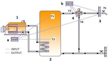
*Figure 1: Hydraulic diagram with control system for domestic hot water preparation.*
