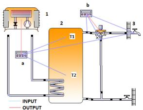
*Figure 2: Hydraulic diagram with control system for domestic hot water preparation with an air-source heat pump.*
