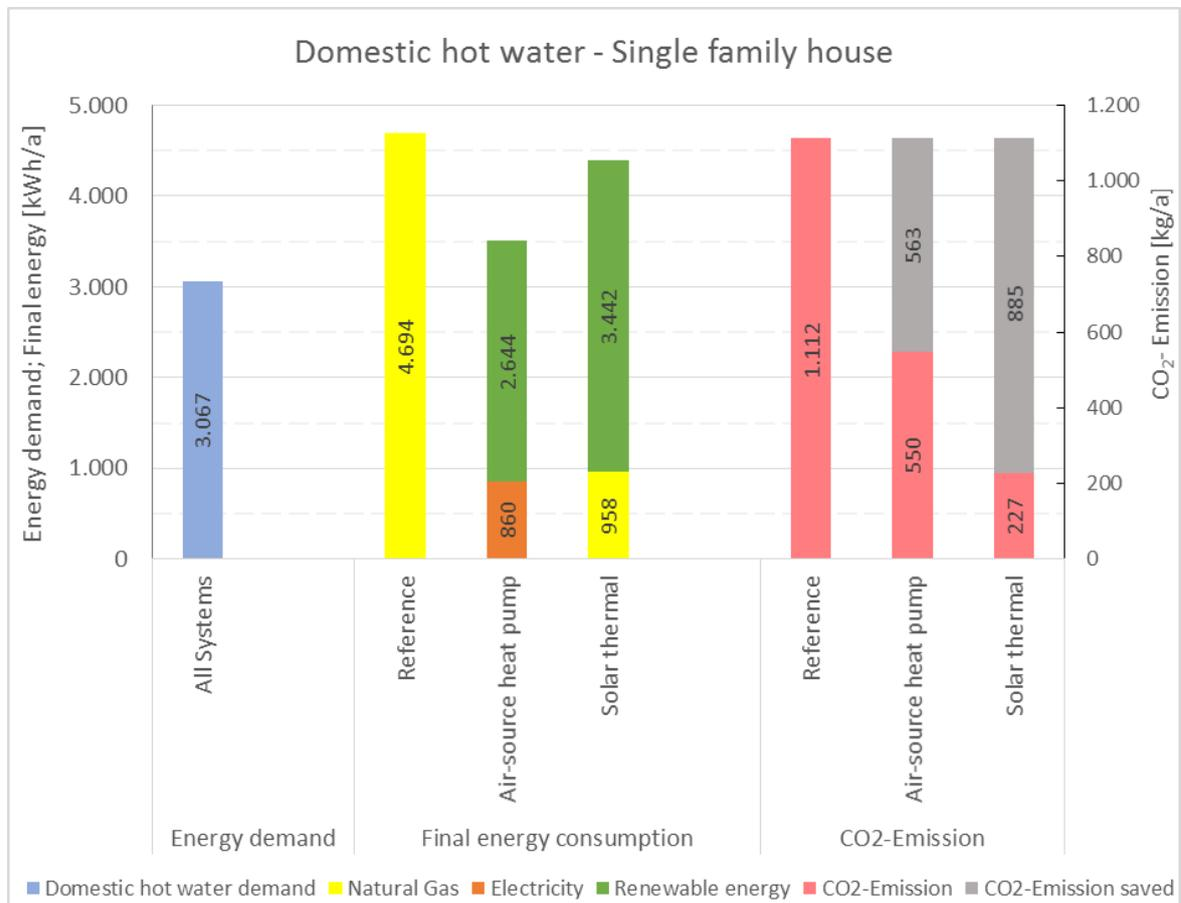
Figure 26: Comparison of all observed heating systems for domestic hot water preparation in single family houses in Madrid.
