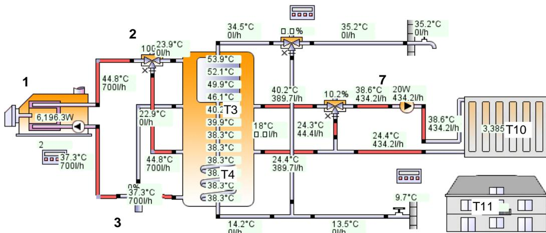
Figure 8: Operation mode space heating.
