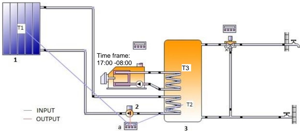
Figure 3: Hydraulic diagram for domestic hot water preparation with solar thermal support.
