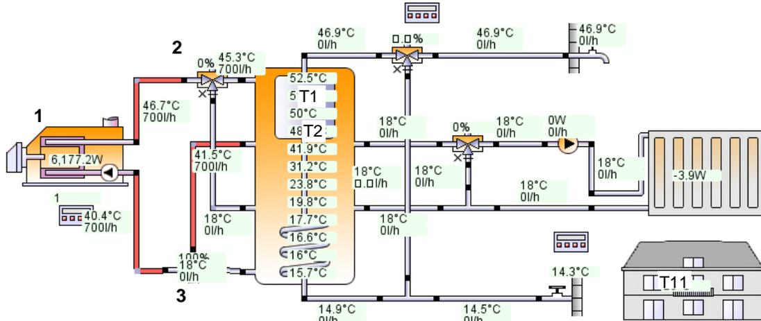
Figure 7: Operation mode domestic hot water.
