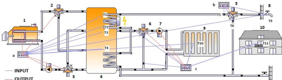
Figure 6: Hydraulic diagram with control system for heating and domestic hot water preparation.
