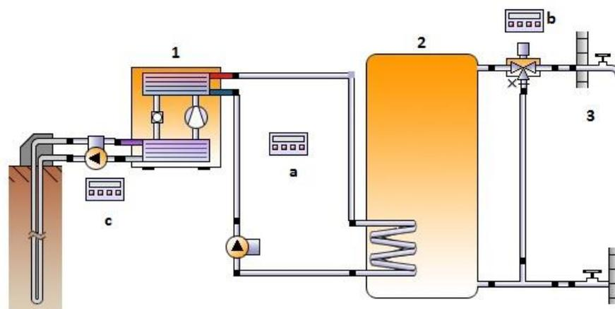
Ground-source loop: 40 mm double U ground loop
