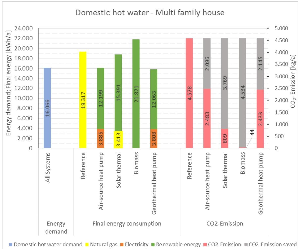
Figure 27: Comparison of all observed heating systems for domestic hot water preparation in multi family houses in Madrid.
