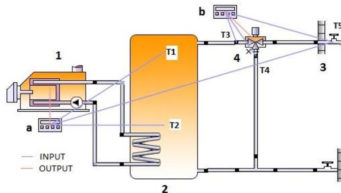
Figure 1: Hydraulic diagram with control system for domestic hot water preparation.
